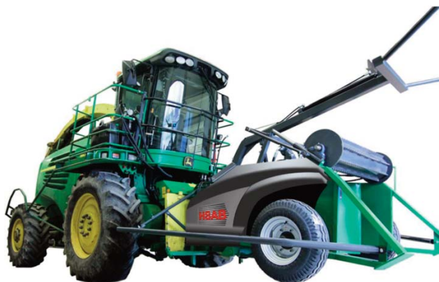
HSAB fully hydraulic head for John Deere self-propelled forage harvester. Image: Nick Parfitt
