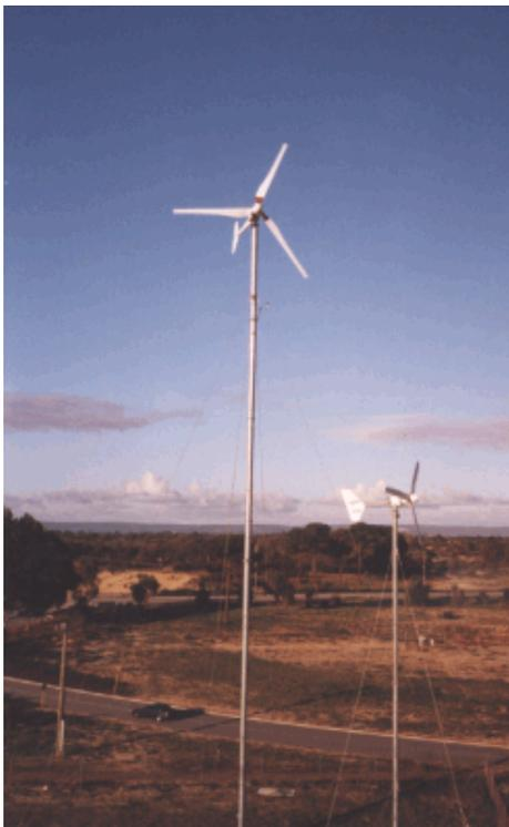
Fig C: Westwind 20kW on 30m mast
