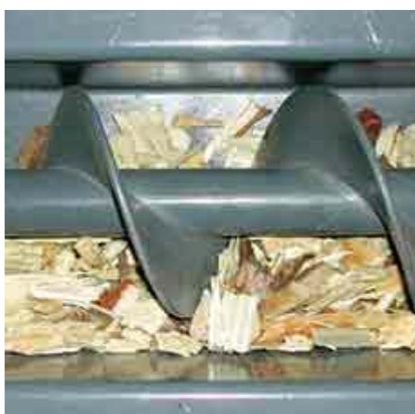
**Figure 13: Woodchip auger screw**
