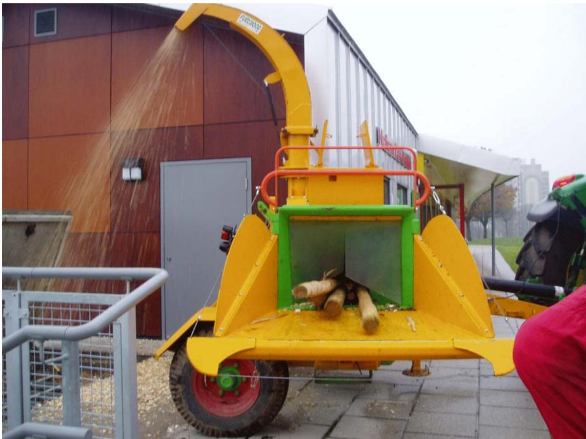
**Figure 3 - Chipper, chipping into a fuel store**
