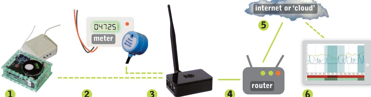
Chariot sensors inside and outside the home collect temperature, humidity and (in some cases) CO<sub>2</sub> data and send to the hub (3)
