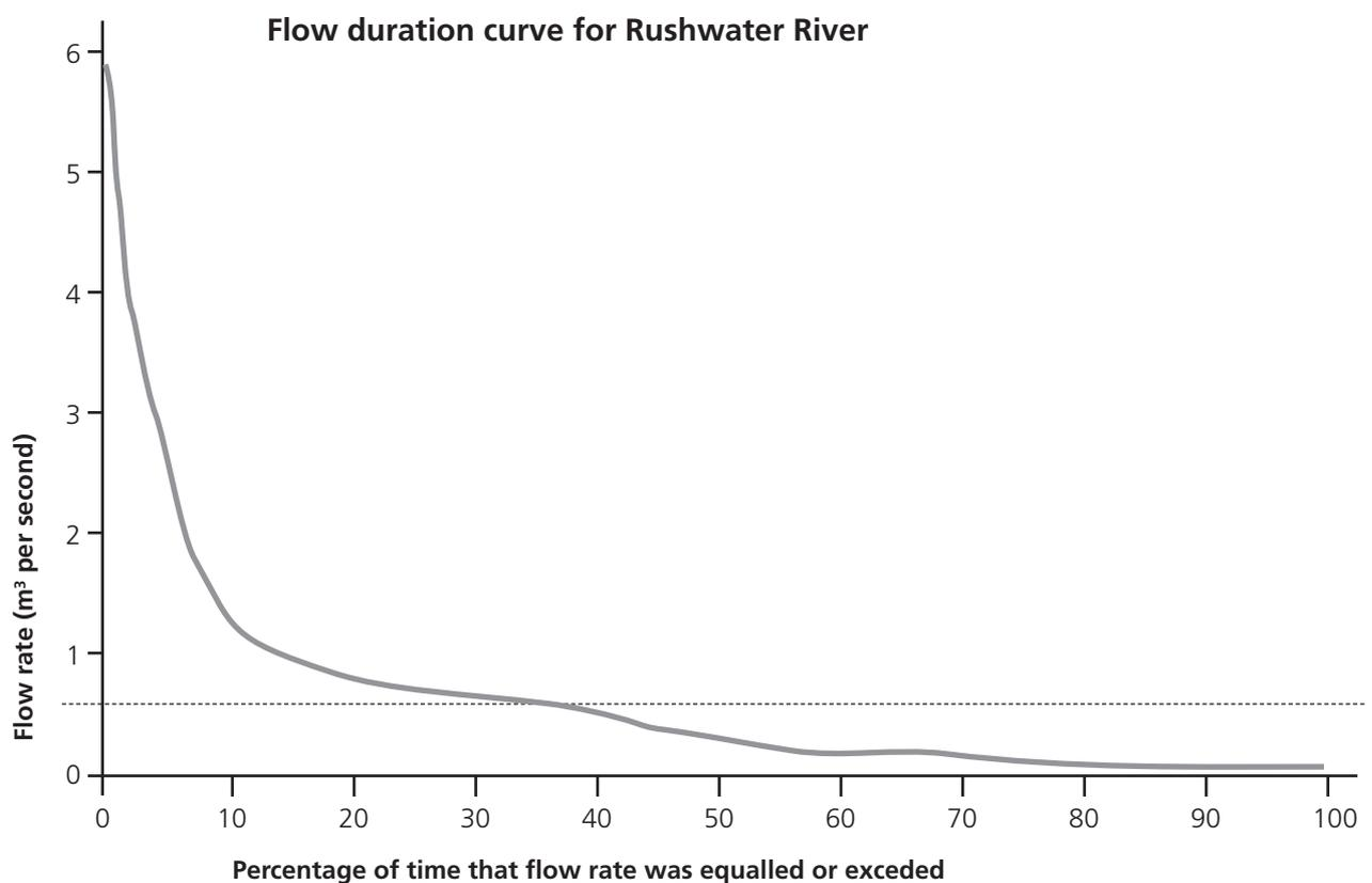
The data indicates that the mean flow rate of the river is 0.53 m<sup>3</sup> per second. They have also concluded that, in order to achieve a decent 'head' of water, a near-horizontal 'leat' (channel) around 150m in length would need to be constructed to channel water from an upstream weir to the 'forebay' tank, from which point an 80m penstock (pipe) would then also need to be constructed to convey the water to the turbine site, creating a total 'head' of 11m.
