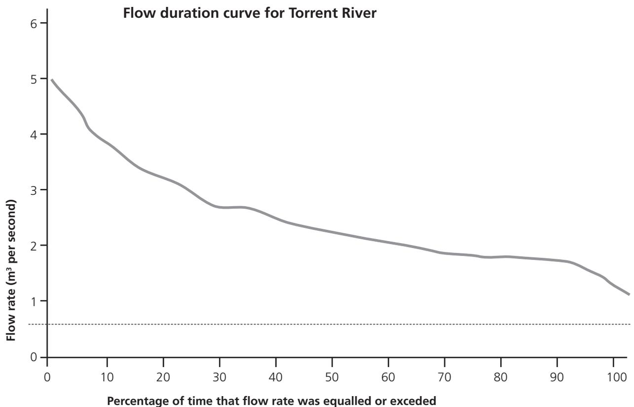
The group has noticed that the maximum flow rate is similar to the Rushwater River site, but that the mean flow rate of the river is 1.85m<sup>3</sup> per second. A refurbishment project would probably re-use the old weir, which has a potential head of around 2.5m, and means that almost no canal or approach pipework is required.
