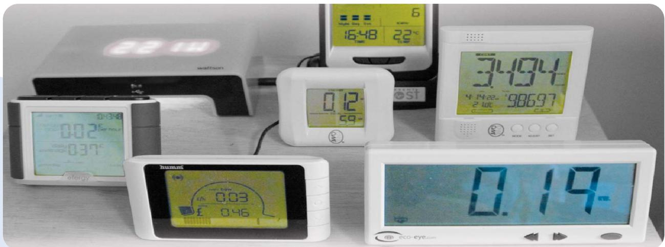
Figure 1: Real-time electricity display devices used in the focus groups - (clockwise from top left) the Wattson, Current Cost CC128 ENVI, Owl, Eco-eye, GEO minim, Efergy lite and (centre) Owl Micro.
