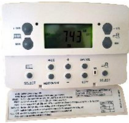
Some new heating controls set the timer and the thermostat together. This lets you set the level of warmth for different times of the day.
