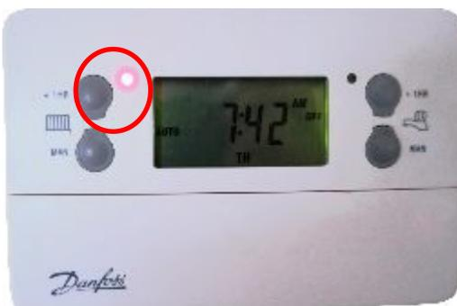
**Advance** moves the heating to the next setting. So if it is off at the moment, it turns on. If it is on at the moment, it turns off.
